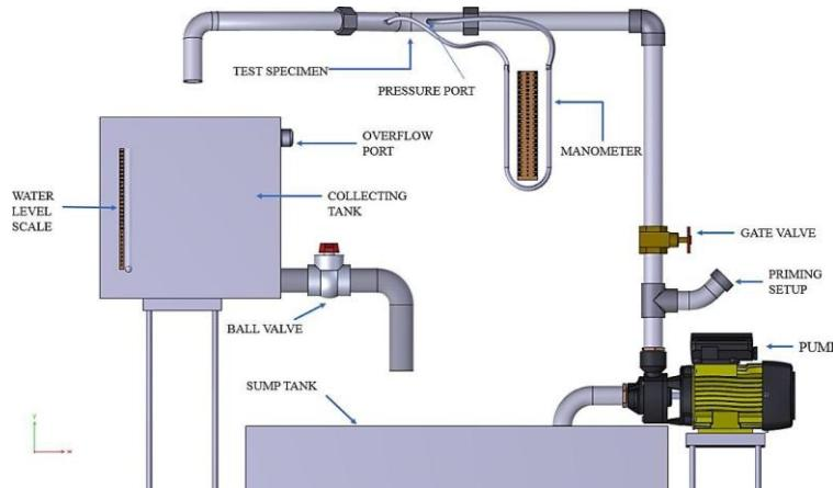
Fig.1 CAD drawing of Experimental setup
