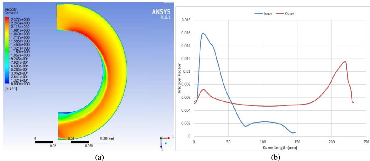
Fig.4. 180RD2 (a)Velocity Contour for 180RD2 (b)Friction Factor v/s Curve Length for Inner and Outer Bend of 180RD2
