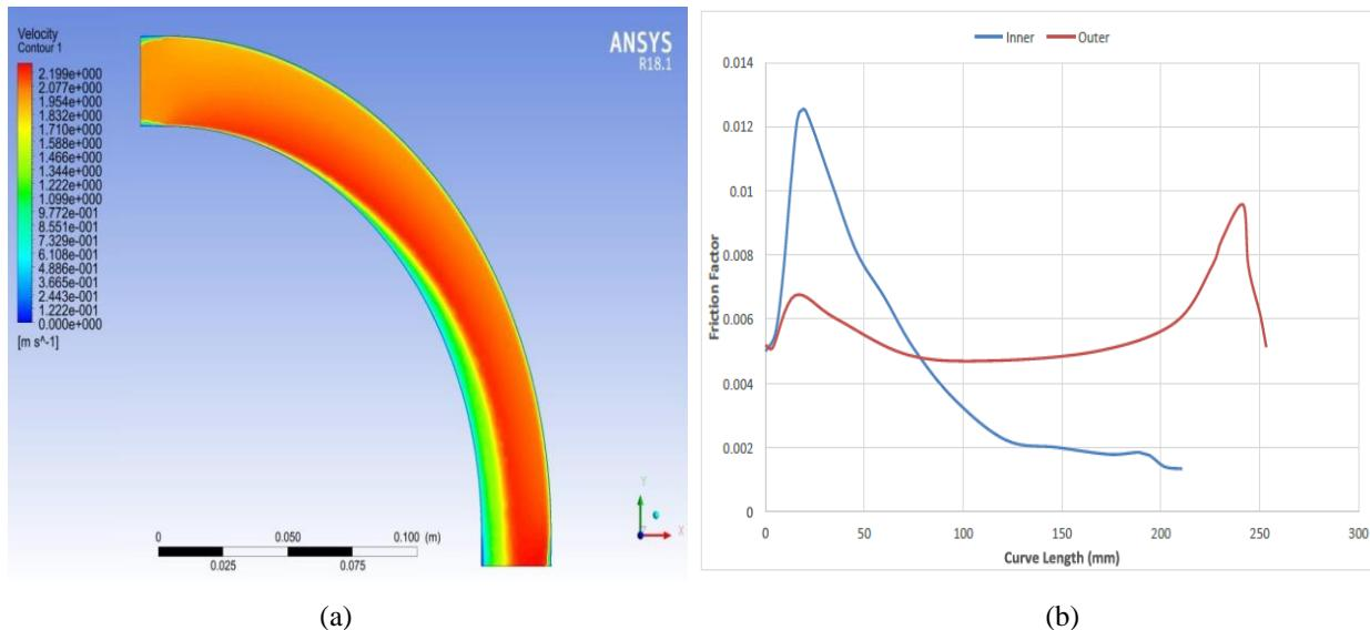
Fig.3. 90RD5 (a)Velocity Contour for 90RD5 (b)Friction Factor v/s Curve Length for Inner and Outer Bend of 90RD5.
