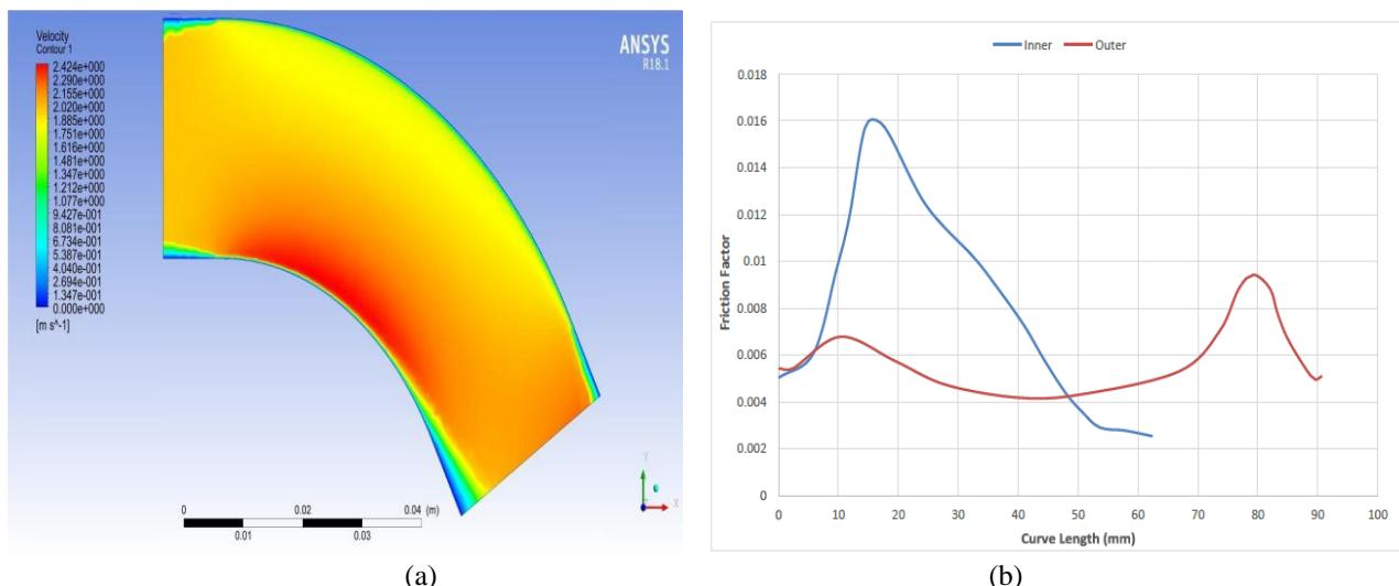
Fig.2.60RD2(a)Velocity Contour for 60RD2 (b) Friction Factor v/s Curve Length for Inner and Outer Bend of 60RD2.
