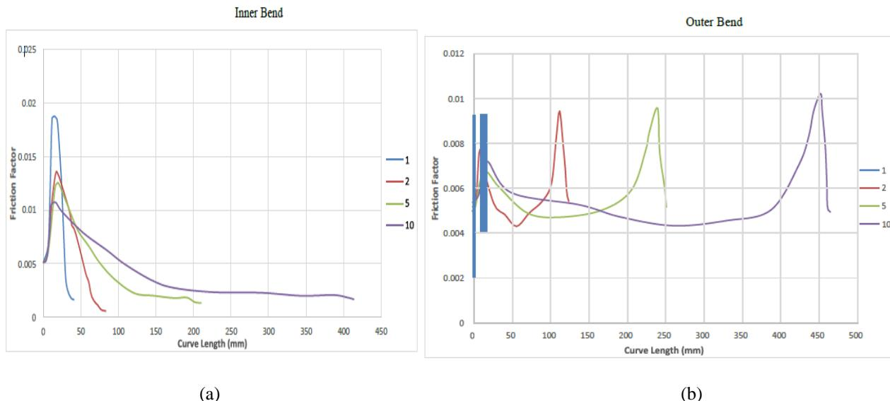
Fig.5.90 DEGREE (a) Friction Factor v/s Curve Length for Inner bend of 90° for different R/d. (b)Friction Factor v/s Curve Length for Outer bend of 90° for different R/d.
