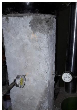
Fig6: NRC2 column Failure
