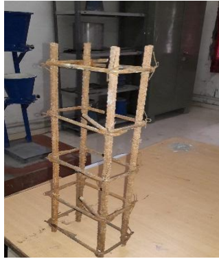
Fig 3: Reinforcement in NRC
