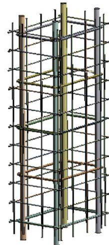
Fig 20: CRC2 Reinforcement Model
