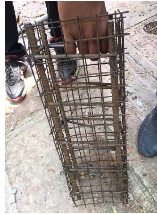
Fig 4: Reinforcement in CRC1(Welded wire mesh 1-inch spacing)
