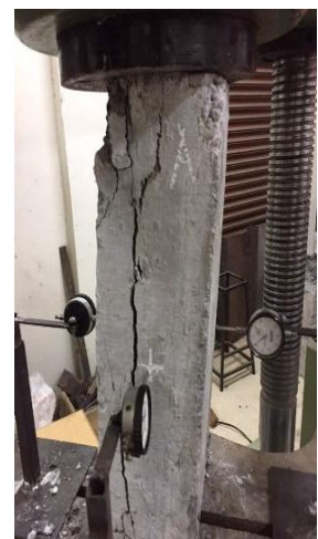
Fig7: NRC3 column Failure
