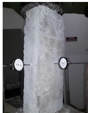
Fig 2: Arrangement of Dial Gauges
