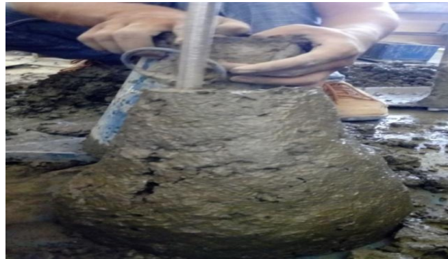
Photo 4.1: Slump Cone Test.
