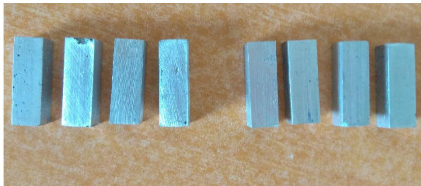
Fig 2. Composite specimens for Mechanical and wear testing
