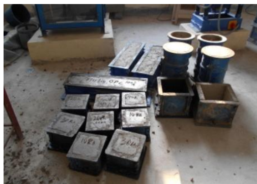
Figure2- Casting of Specimens
