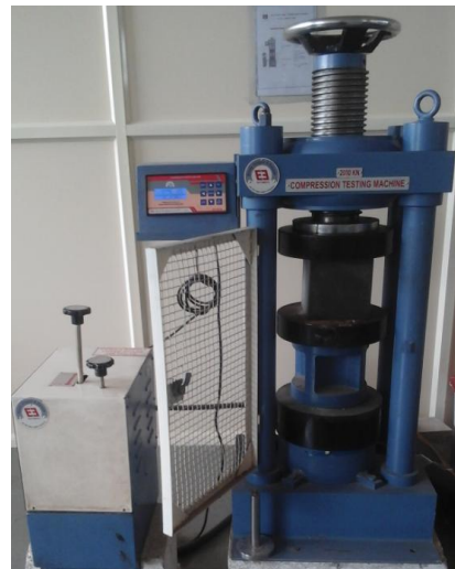
Figure 9- Testing of Cube for compression test
