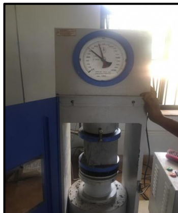
Fig 5: Compression test on cube specimen
