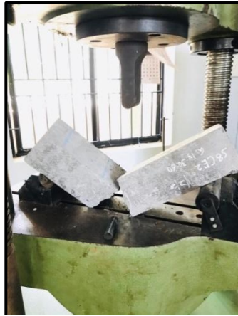
Fig 9: Flexural strength test on beam specimen
