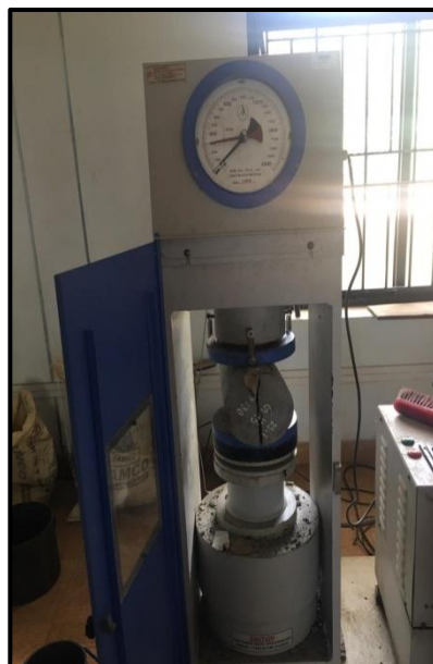
Fig 7: Split tensile test on cylindrical specimen
