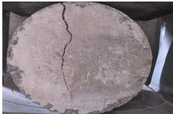
Fig. 3. Failure Pattern of Cylinder
