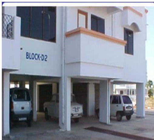
Figure 1.1 Vertically irregular buildings
