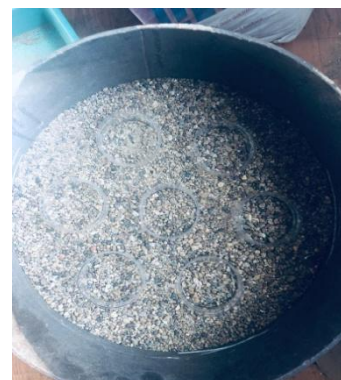
Fig 3: Placing of flex cell
