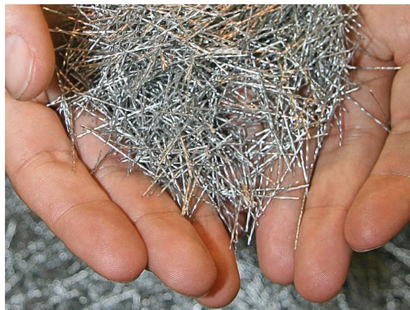
Fig- 2.2: sample of steel hook fibres used in concrete
