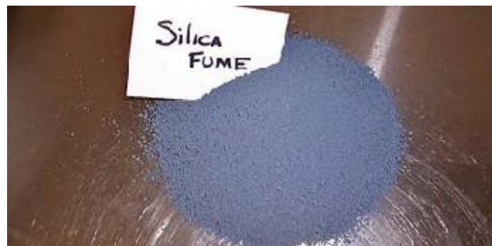
Fig- 2.1: sample of silica fume used in concrete
