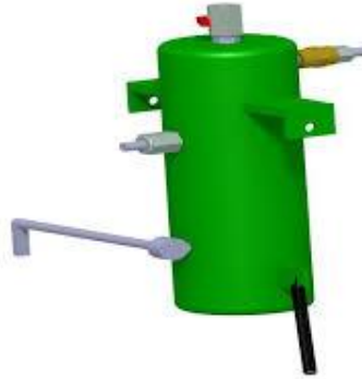
Fig 3 3D image of Mixing Chamber
