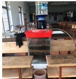
Fig.1. Filtration process in vermifiltration model
