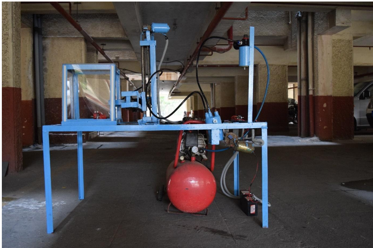
Figure 2: Assembled front view of the abrasive jet machining equipment
