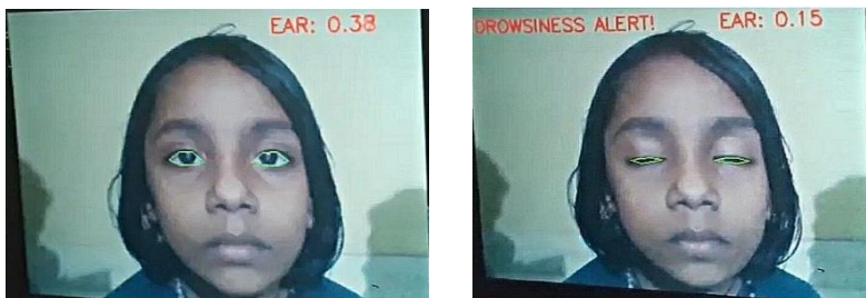
FIGURE 6: TEST 2(A) EYE DETECTION (B) DROWSINESS DETECTION
