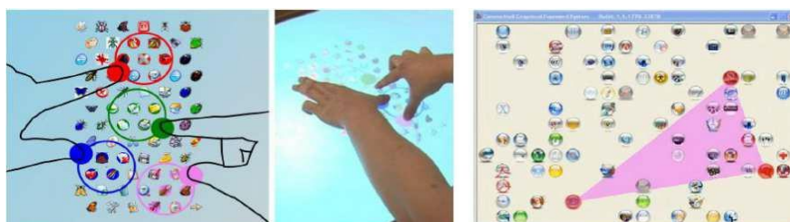
Figure 3. (a) Color Rings method [25]. (b) Convex Hull method [36].
