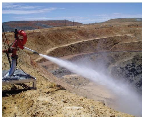
Fig. 6. picture showing chemical suppressant
