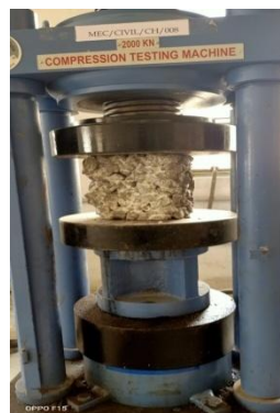
Fig. 2: compressive strength test for specimen cubes.
