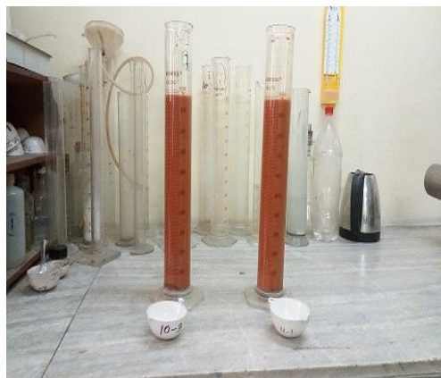
Fig 1. Test Set-up for mechanical analysis by pipette method
