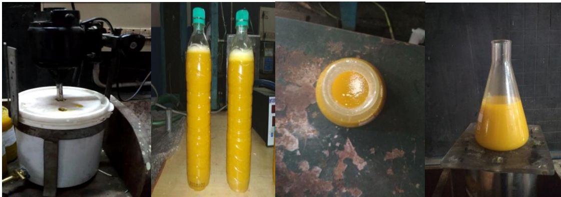
Fig2: emulsion and nano emulsion a) mechanical stirrer b) Mahua emulsion c) and d) Nano Emulsion
