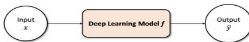
Fig. 2: High-level illustration of deep learning model f . Generally, a single input instance x generates outputs y^- . No other metadata or explanations are generated other than the output classification. Most model inference scenarios involve this method where model f is considered as a blob of information which takes an input x and generates an output y^- .
