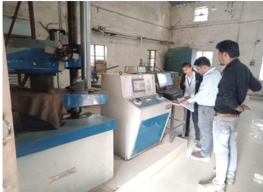
(a) (b) Fig.No.3. compressive testing of zeolite powder replacement with cement having size of cube 150 *150 *150mm and it is tested on universal testing machine whose least count is 1 N/mm 2 after 7 and 28 day curing..
