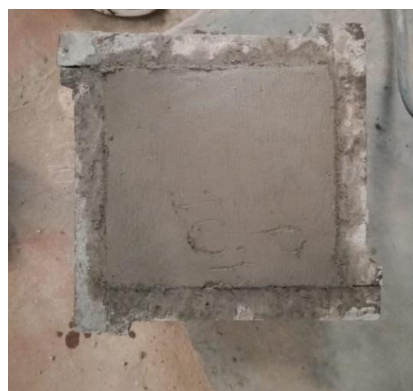
Fig.No.2. In above figure, 15% replacement of zeolite powder with cement block was been seen.
