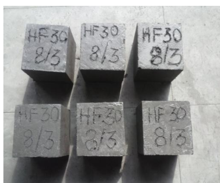
Fig 12: cube specimen before acid attack
