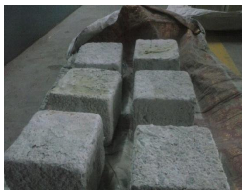
Fig 13: cube specimen after acid attack
