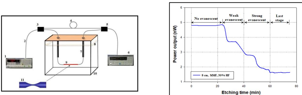
Fig. 4. Optical output power vs. etching time using 30% HF solution.
