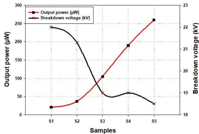
Fig. 8. Characteristics of output power and breakdown voltage.
