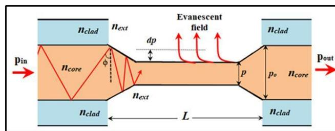
Fig. 1. Cross section of the sensing arm
