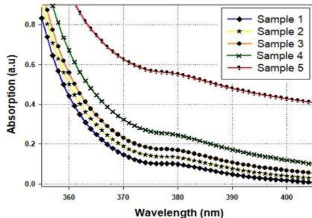
Fig. 9 Absorption spectrum signal of transformer oil samples
