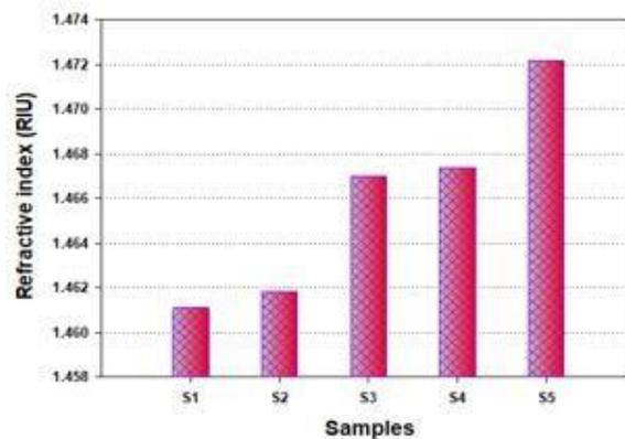
Fig. 6. Refractive index of oil samples at 24 °C.
