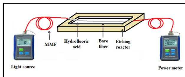
Fig. 2. Schematic diagram of setup for etching process.
