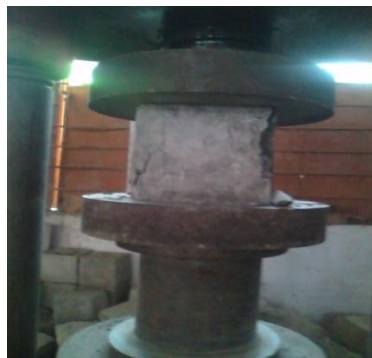
Fig . 2: compressive strength test for specimen cubes.
