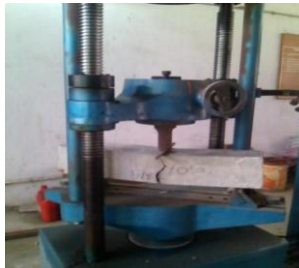
Fig. 4: Testing on beam
