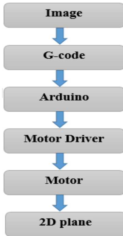
Fig. 1 Block diagram of CNC Plotter
