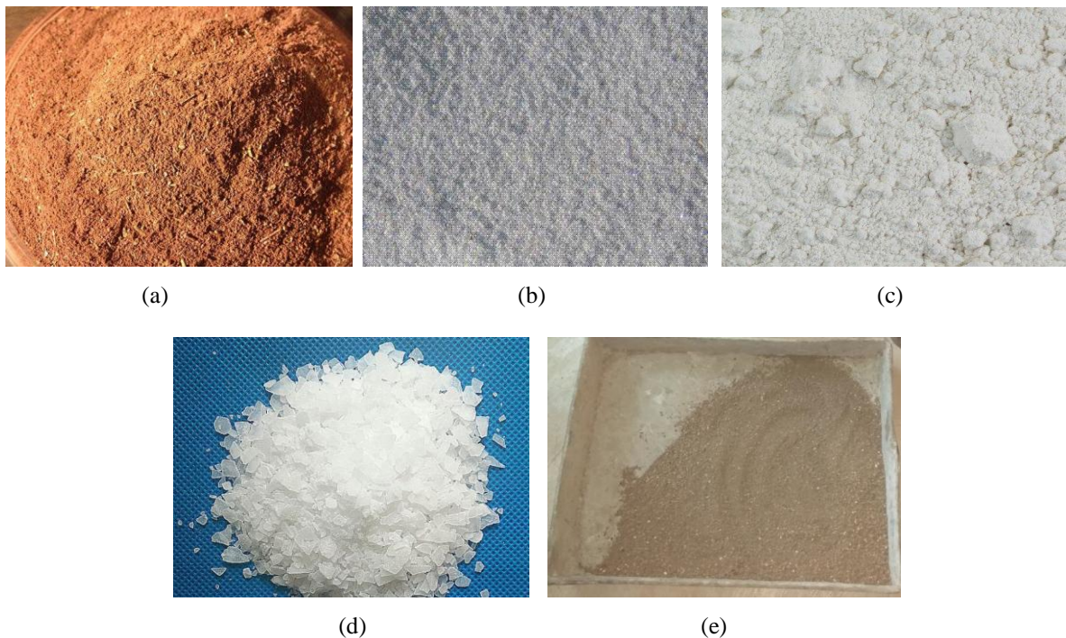
Fig. 1 Material used (a) Brick powder (b) Marble powder (c) Fly ash (d) Magnesium chloride (e) Soil
