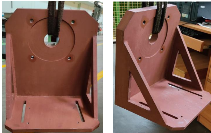
Figure 5: Fabricated 6.2kW Motor Fixture
