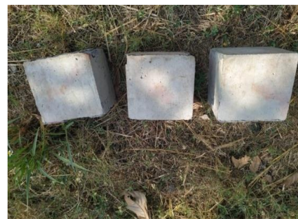
Figure 4:- Modified self cleaning cube sample kept under sunlight after 24 hours
