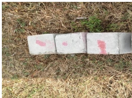
Figure 3:- Normal cube samples kept under sunlight after 24 hours
