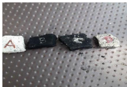
Figure 5:- Mortar cube samples used for EDAX test
