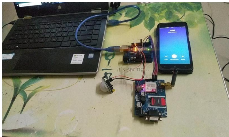
Fig. 10. Snapshot of the work with a call is successfully generated by GSM module
