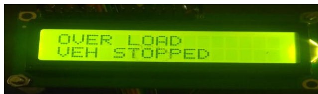
Fig.6 The output when the vehicle is overloaded at the steps and the motor is set off respectively.
