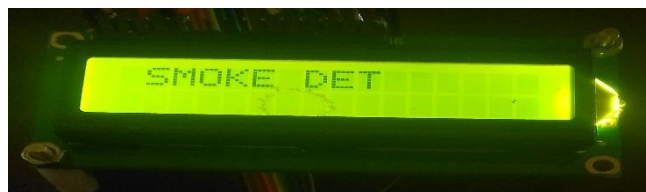
Fig.8 smoke is detected and message is sent to the user.
