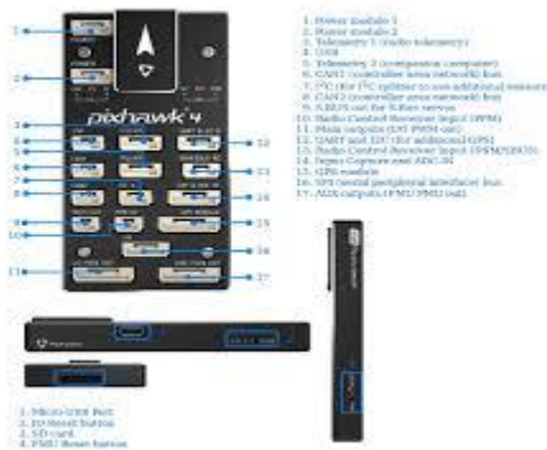
fig:7 :pixhawk ports
