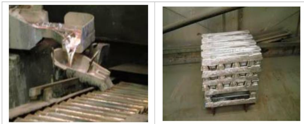
"Fig. 1" The casting process of metal aluminum produced from dross reprocessing [5]
