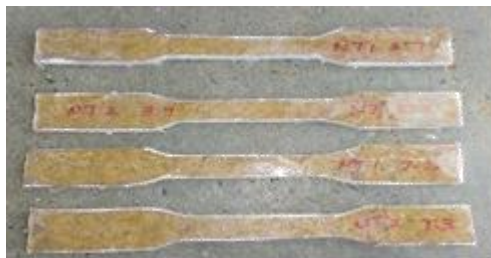
Fig 2 Tensile test specimens
