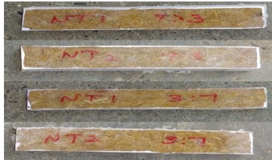
Fig 4 Flexural test specimen
