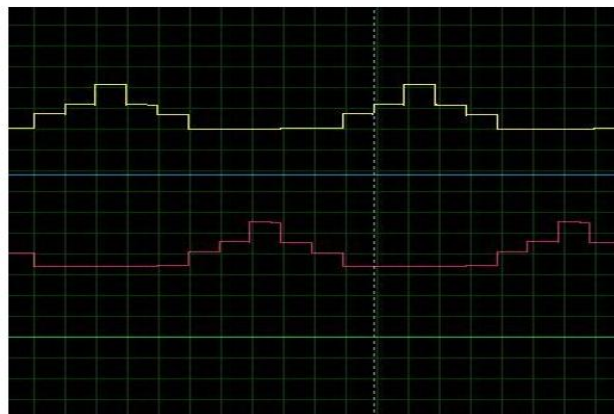
Fig4. A,C - Five step output wave forms of voltage divider network
