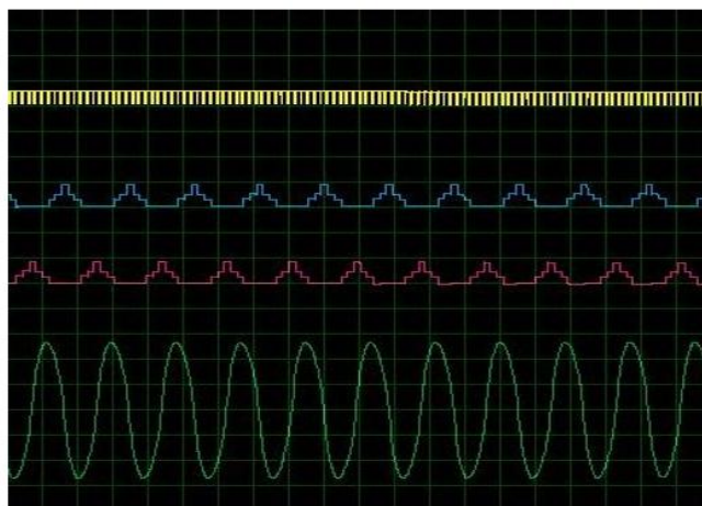
Fig5.A Clock signal, B, C- five step output waveforms of voltage divider network
