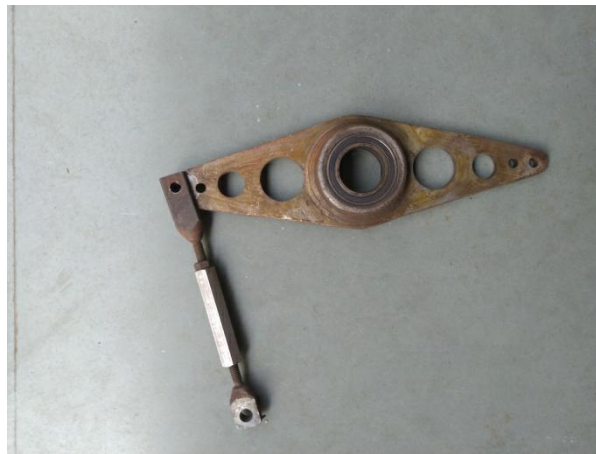
Fig. 02 Drivetrain mounts with turnbuckle
