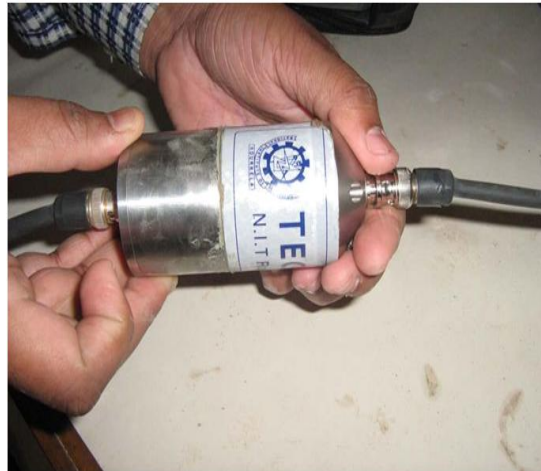
Fig. 04 Zeroing of the Transducers Following table shows ultrasonic pulse velocity calibration tests carried of 6 samples along with compression test results.
