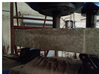
Figure 3.2. Flexural test on Bubble deck slab
