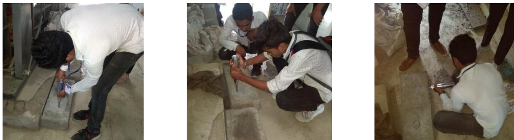
Figure 4.3. Test Performance of rebound hammer
