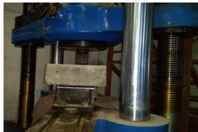
Figure 3.1. Flexural test on conventional slab
