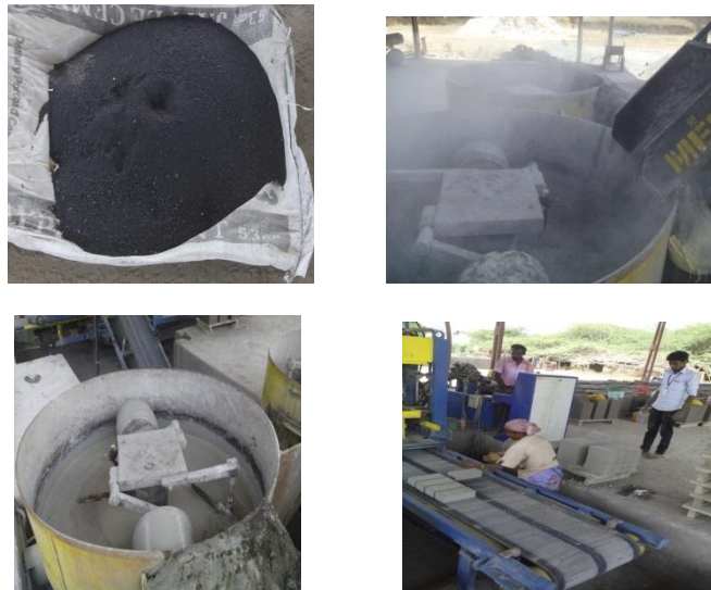
Fig 3. Casting of Fly ash bricks with Steel mill scale through wire cut machine.
