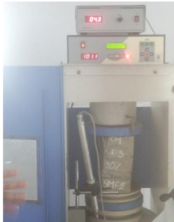
Fig 11 Triplet prism test on Steel mill scale in Fly Ash bricks
