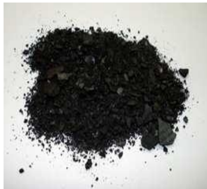
Fig 1. Before grinding of steel mill scale
