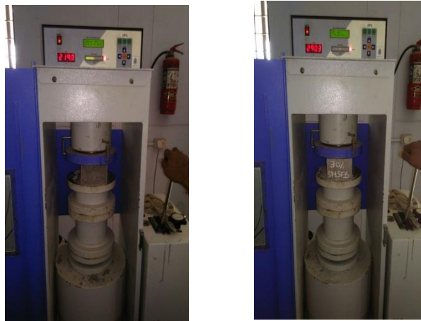
Fig : 4.(a) Testing of bricks
