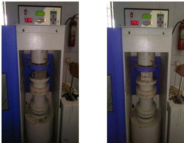
Fig : 4.(b) Testing of bricks
