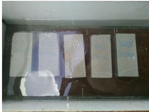
Fig: 5. Water Absorption Test For Various Mix Proportioning Of Steel Mill Scale
