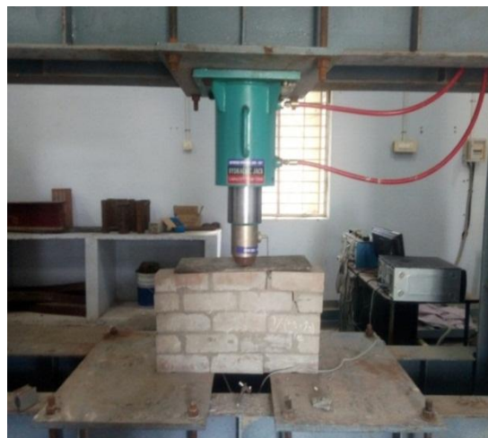
Fig 14 Wall Panel Test
