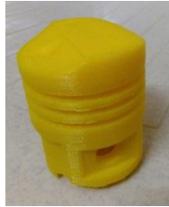
Fig 3. Prototype of piston generated by rapid prototyping
