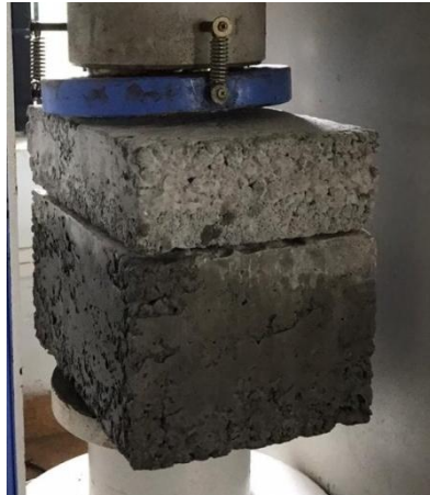
Fig 3: Compression test on lego model building block
