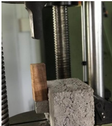
Fig 4. Shear test of the projection of lego model building block
