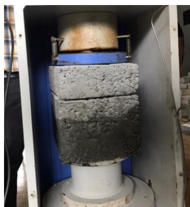
Fig 7 Compression Test on Lego Model building block
