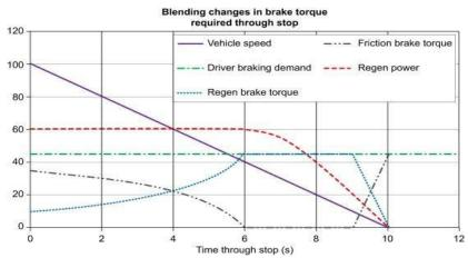
This graph shows the blending changes in brake torque required through stop with regards to how every single parameter affect the brake torque.
