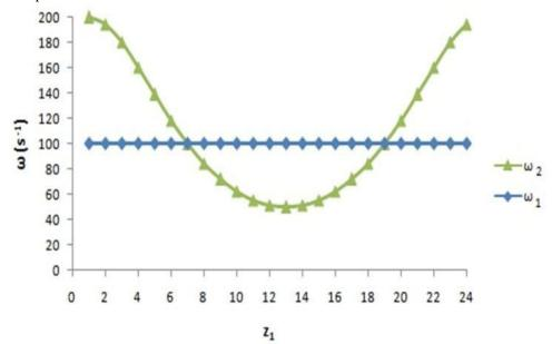
The rotational speed on drive wheel gear and driven wheel gear is constant to standard spur gears (Blue line). The graph varies for designed elliptical gearing with variable transmission, the angular velocity of the driven wheel is not constant but varies according to continuous changing of the gear ratio (Green Line).
