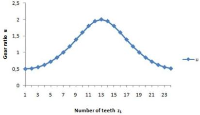
The above graph shows the correlation between the number of teeth present on the spur gear and the gear ratio. This is a course of continuously changing gear ratio. A gear ration value less than 1.0 indicates overdrive and gear ratio greater then 1.0 indicates speed reduction.
