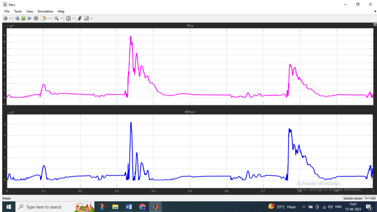
Fig. 6 DC link Capacitance voltage
