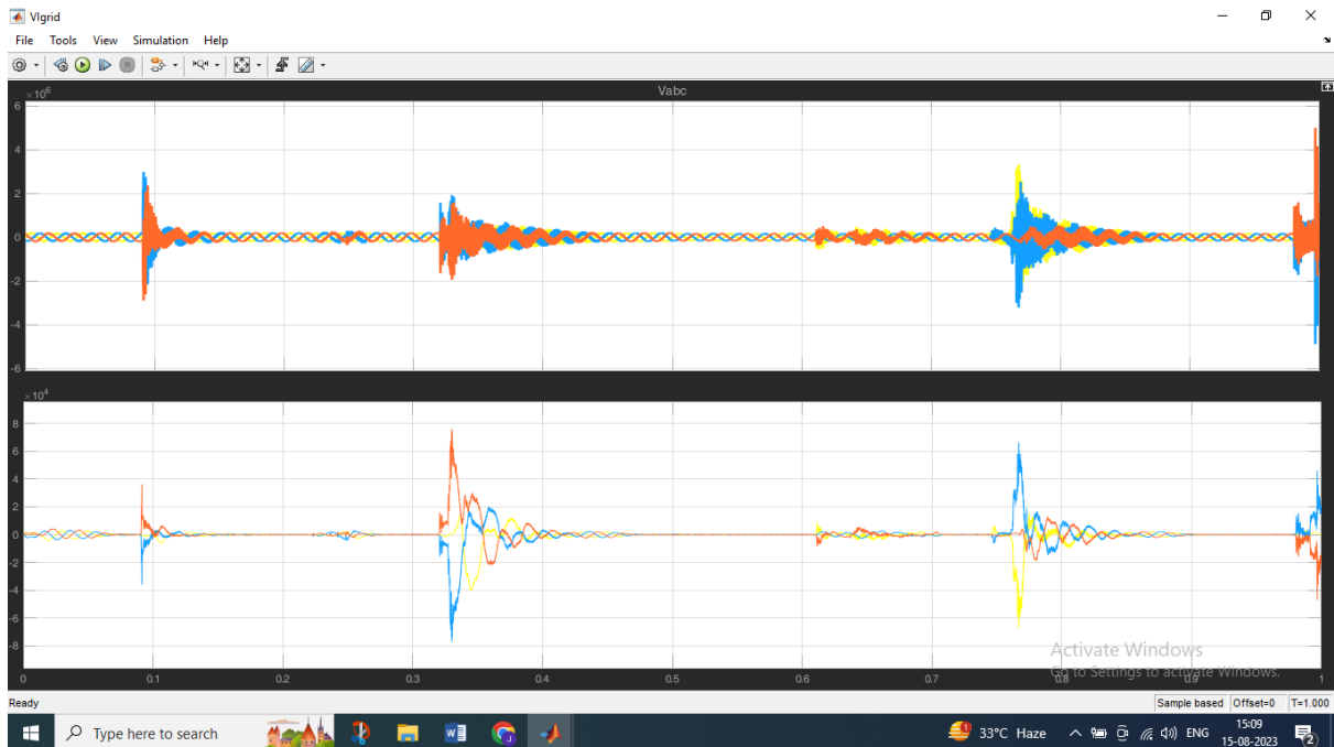
Fig. 7 Three Phase Grid Voltage Vgrid and Grid Current Igrid
