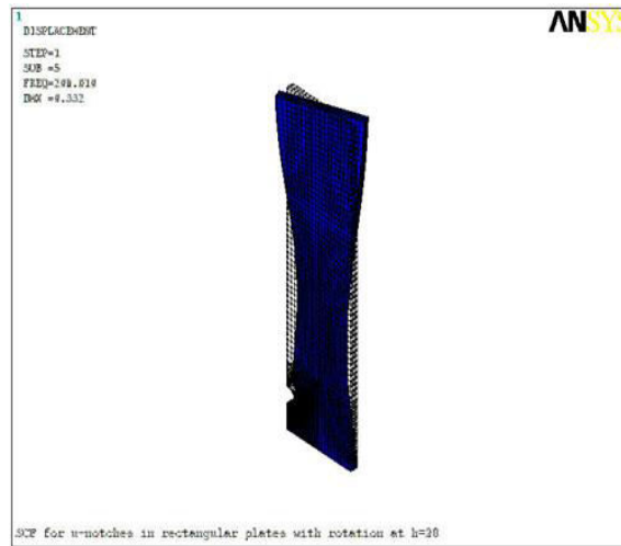
Figure 7: 1T mode of rectangular blade with semicircular notch at h = 20mm
