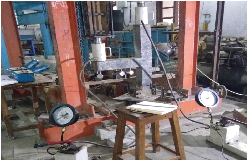
Figure 1: Monolithic Connection placed on Moment Frame
