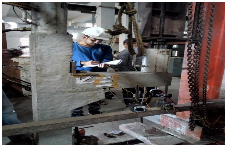
Figure 2: Dry Precast Connection placed on Moment Reaction Frame
