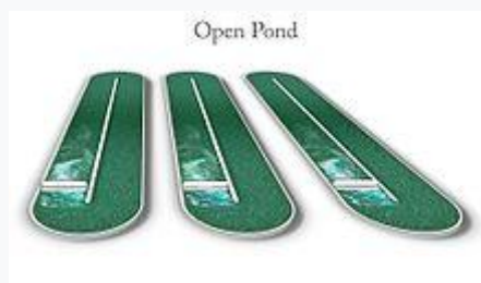
Design of a race-way open pond commonly used for algal culture
