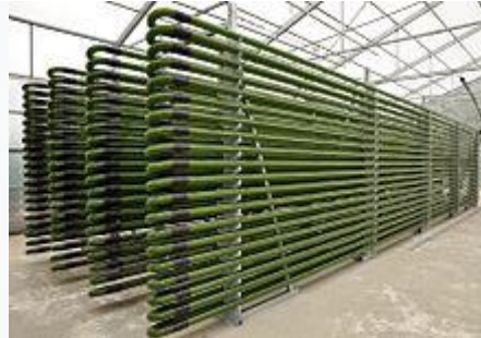
Photobioreactor from glass tubes
