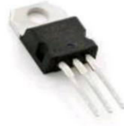
Fig: Voltage regulators
