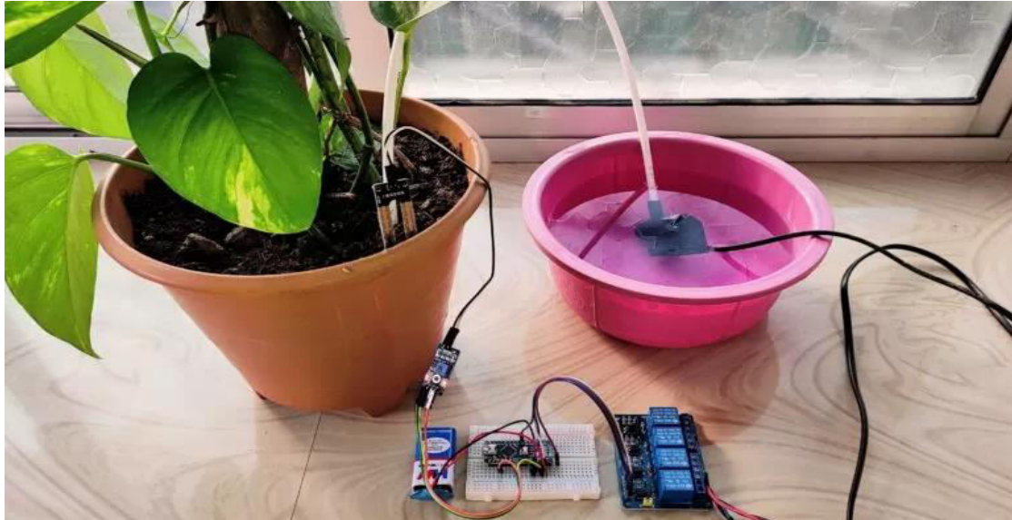
Fig.2. Temporary Working Module of Automated Plant Watering System.
