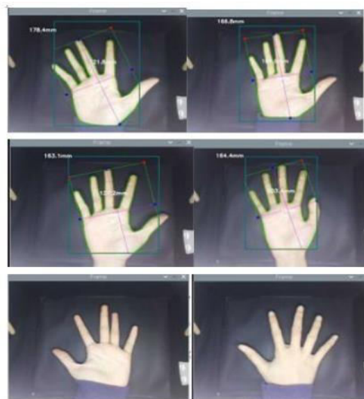
Fig. 4. The results of hand palm detection and area measurement
