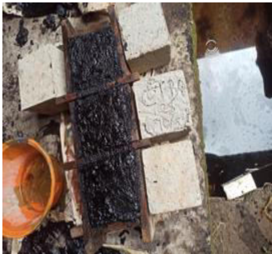
Plate 3: after placing concrete in cubic moulds
