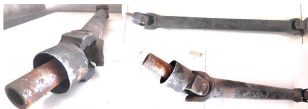
Figure 2. Drive Shaft for Case Study
