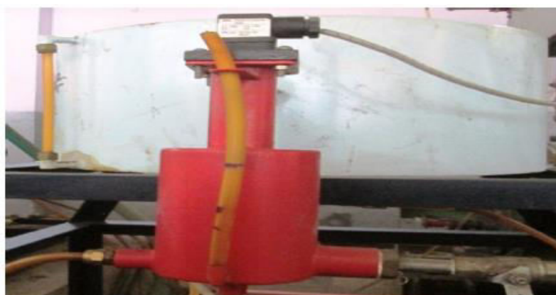
Figure 2: Fuel Consumption unit
