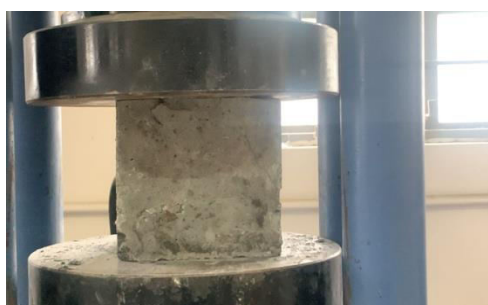
Fig. 1: Testing of cubespecimen in CTM
