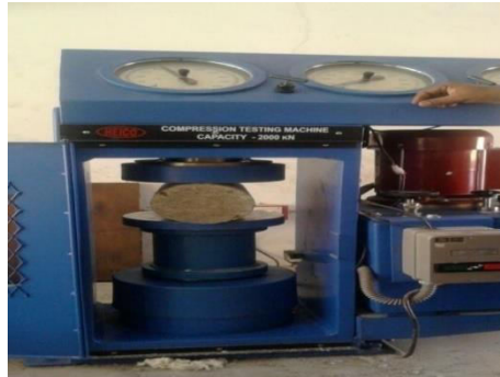
Fig. 2: Testing of a sample in CTM
