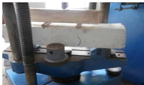
Fig.4: Propagation of crack under the roller
