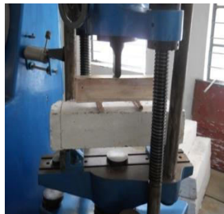
Fig.3: Loading of beam specimen
